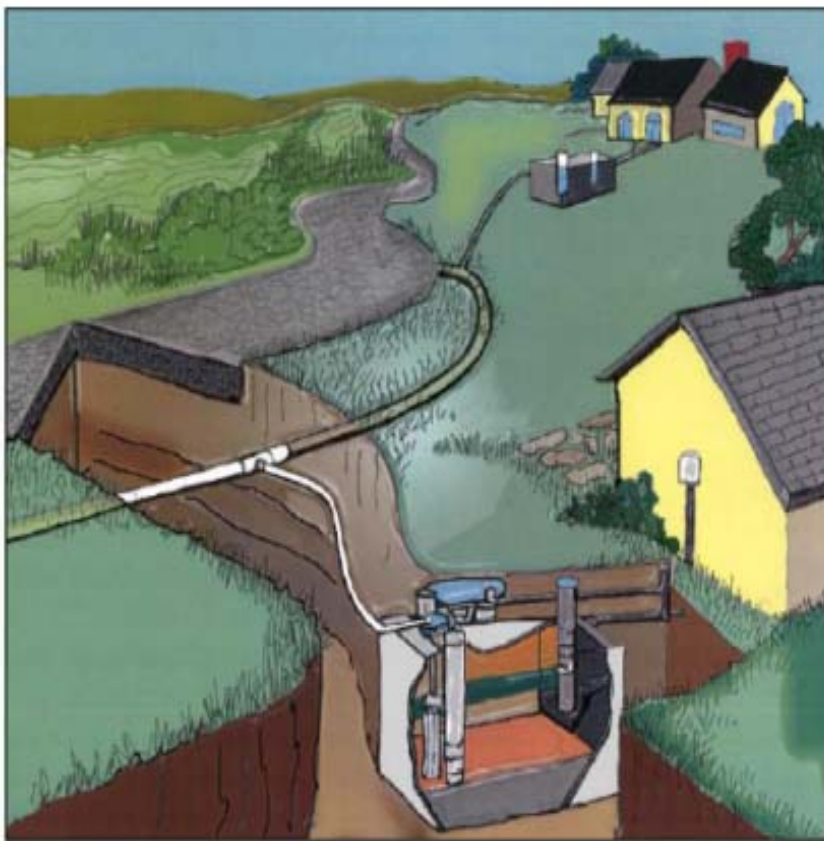
STEP systems use septic tanks to remove larger solids and small pumps to transport the sewage effluent.
